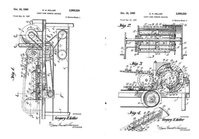
Drawings used in Fr. Gregory Keller's 1960 patent application for a machine to place the hook in candy canes (Courtesy of Arkansas Catholic)
