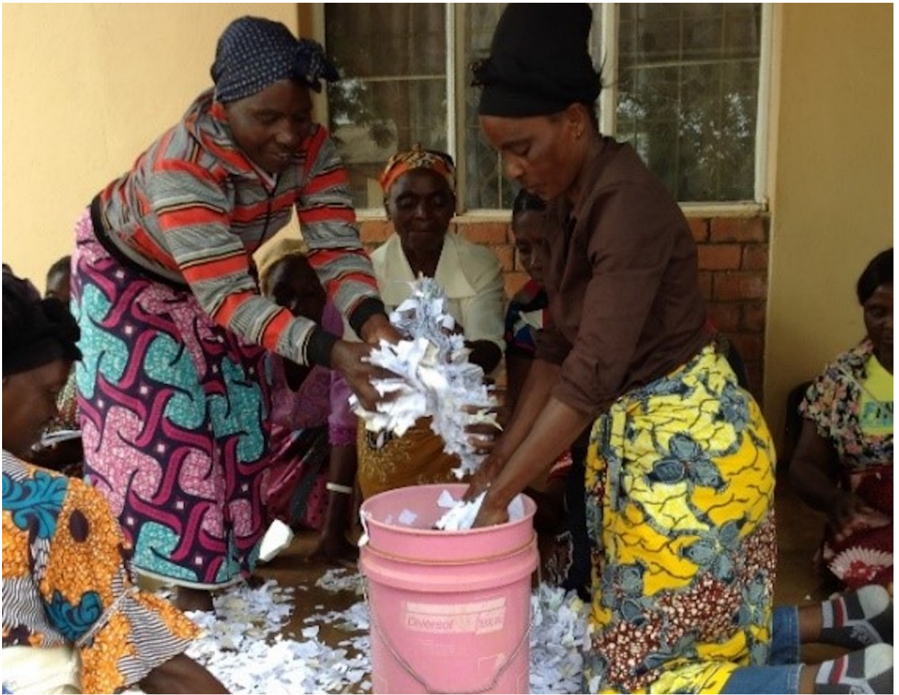
Women soak the shredded paper for up to a week to make a paste. (Provided photo)
