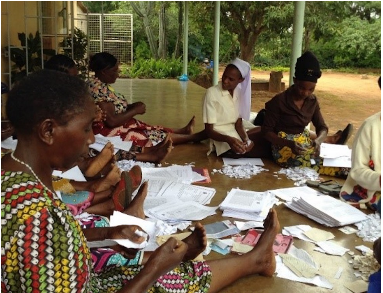
The process of making paper charcoal begins with shredding paper into small pieces. Holy Spirit Sr. Edna Himoonde, in white habit, sits with the women of Chikuni shredding collected paper. (Provided photo)
