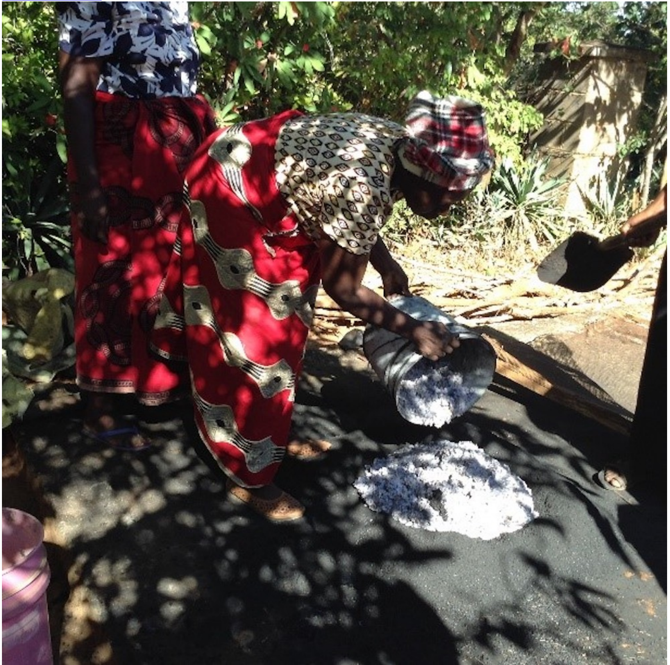
A woman in Chikuni, Zambia, adds paper paste to the corn cob ash. The mixture will be formed into balls and dried into a burnable fuel alternative to charcoal from trees. (Provided photo)
