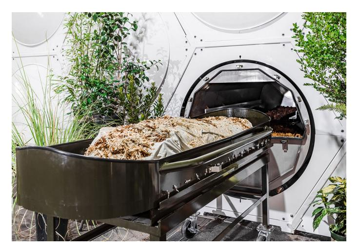
An example vessel that is used in the natural organic reduction process, which converts human bodies into soil, created by Recompose. (Courtesy of Recompose/Sabel Roizen)
